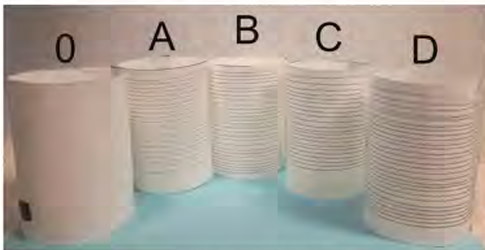
Figure 2. The photo shows pure cellulose fibres (0) and GO/CEL composite fibres (A–D). The obtained fibres look identical, regardless of the coagulation method (water-1; methanol-2).
